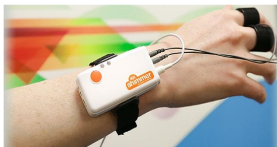
Figure 3. Close-up view of the Shimmer 3 GSR+ device used for recording Electrodermal Activity (EDA) (Source: https://shimmersensing.com/ ).
