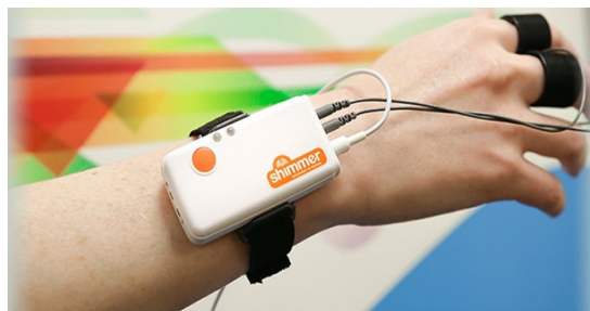
Figure 4. Close-up view of the Shimmer 3 GSR+ device used for recording Electrodermal Activity (EDA) (Source: https://shimmersensing.com/ ).
